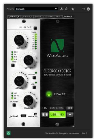
The VST/AAX plug-in can send automation to and receive it from the hardware via USB, with both reflecting the change in settings.
