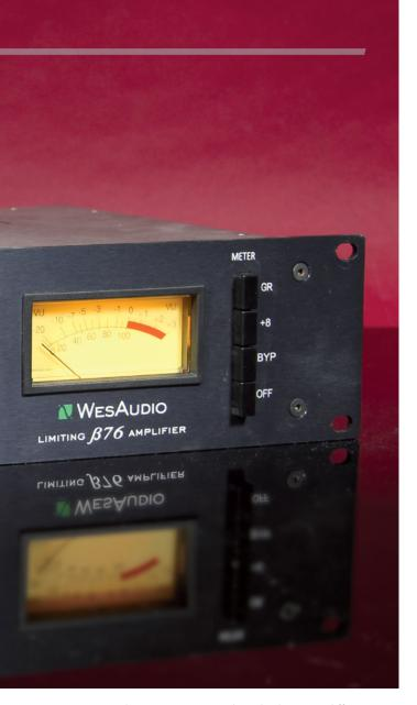
On closer examination, though, there are differences. First off, there's a side-chain filter, which is switched in and out and governed by a single button, which in turn controls a relay switch. This allows you to roll the bottom end off the control signal at 60, 80 or 150Hz, which is a useful touch. Essentially, it allows you to let through energetic low frequencies without triggering compression.
