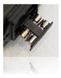
A spare fuse is included in the power supply, allowing you to quickly swap it with the primary fuse when needed.
