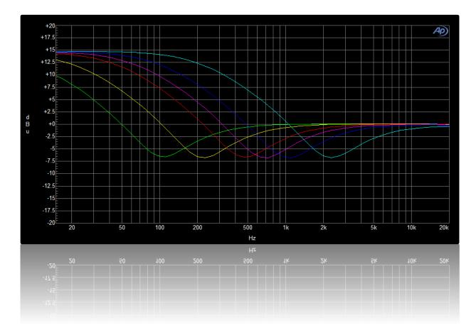
Graph shows all possible frequency ranges: 20, 30, 60, 100, 120, 250 (Hz) and maximum BOOST and CUT values set at the same time.
