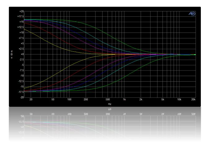
Graph shows all possible frequency ranges: 20, 30, 60, 100, 120, 250 (Hz) and maximum BOOST and CUT setting respectively.
