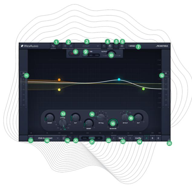
In Stereo mode, the Stereo plug-in shares the same controls as in Dual and MS modes. The key difference is that Stereo mode consolidates the interface to display only one channel. This visible channel functions as the master, automatically synchronizing both hardware channels to the same settings.
