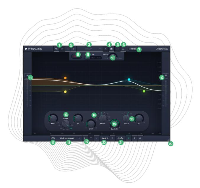
The layout of the mono plugin closely mirrors that of the hardware, maintaining the intuitive interface and design of the 2-channel stereo plugin version. However, there's a notable difference: the unit mode buttons (DUAL / STEREO / MS) are absent in this configuration. This is because, in mono plugin mode, the \_PROMETHEUS automatically operates in DUAL unlinked mode, optimizing it for independent channel processing.
