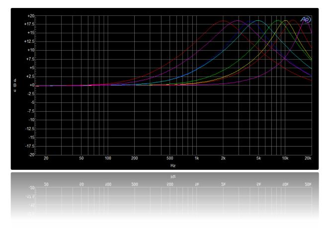
Graph shows all possible frequency ranges: 2, 3, 4, 5, 8, 10, 12, 16 (kHz) and maximum BOOST setting.
