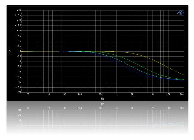
Graph shows all possible frequency ranges: 4, 8, 12, 20 (kHz) and maximum CUT setting.
