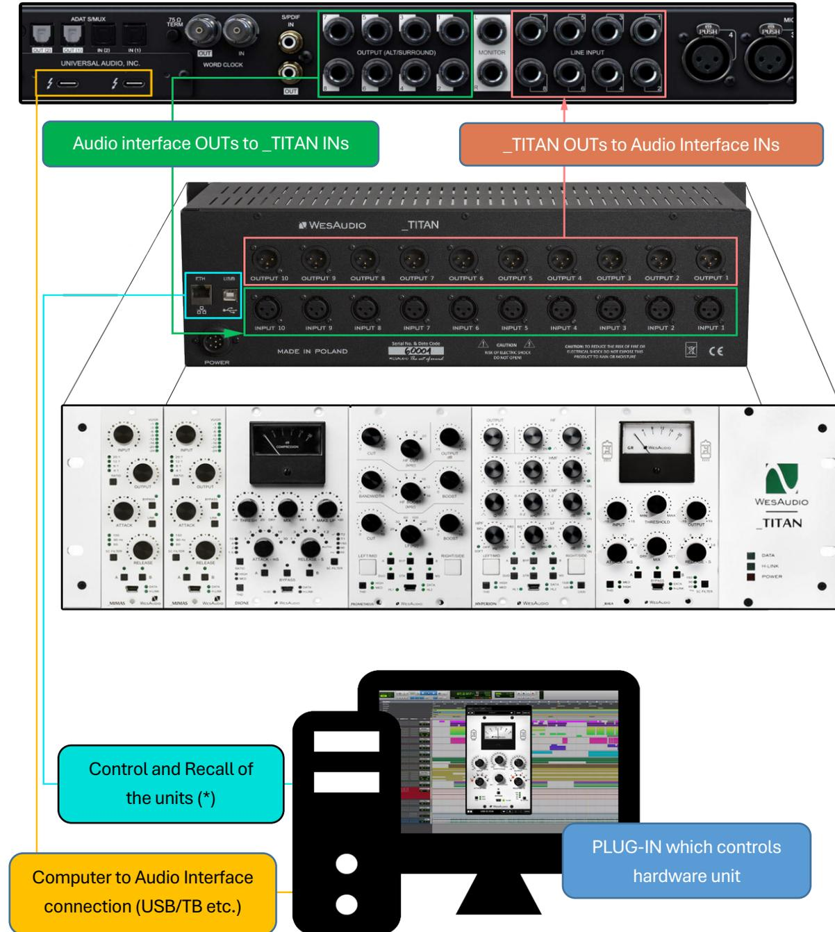
(\*) Please note that \_TITAN Ethernet connection doesn't require direct connection with the PC/MAC – You can also plug in the \_TITAN directly to the router and use your local network to access and control all units inside \_TITAN.
