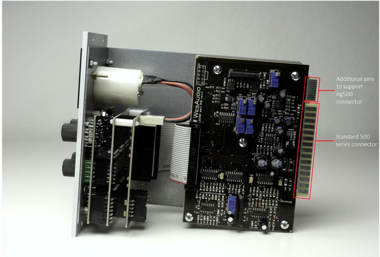
This extension is designed to work with the standardized plug type in the 500 series. Yet, some manufacturers use large screws on the plug, hindering device compatibility. Research indicates that over 90% of 500 series racks are compatible. For more information, please visit: <https://wesaudio.com/ng500/>.
