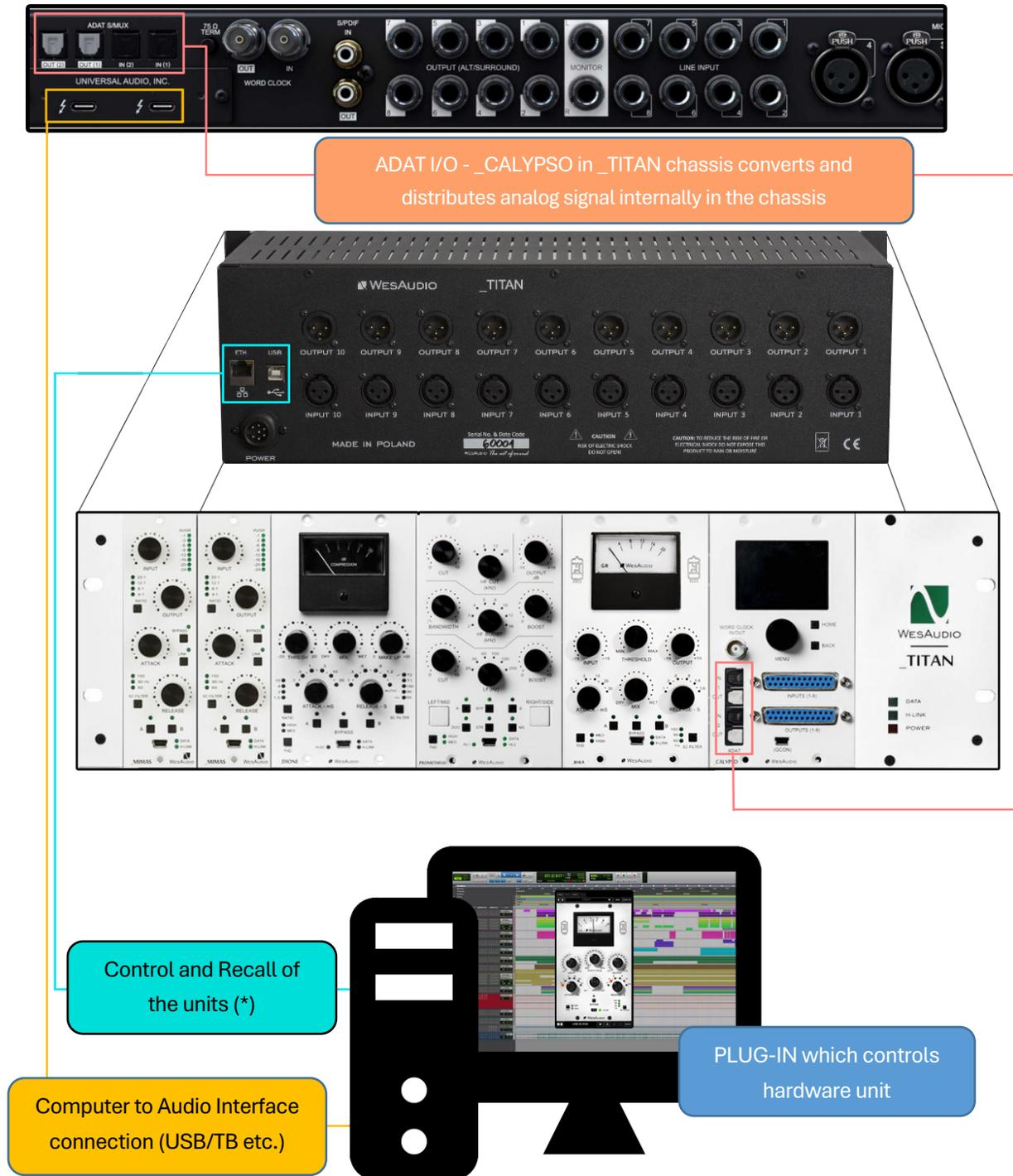
(\*) Please note that \_TITAN Ethernet connection doesn't require direct connection with the PC/MAC – You can also plug in the \_TITAN directly to the router and use your local network to access and control all units inside \_TITAN.
